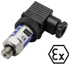
The BCX series is an ex-proof pressure transmitter designed for use in hazardous areas with a risk of explosive atmospheres. Operating on the piezoresistive principle, this series can be safely used in applications involving various fluids such as water, air, and oil.
