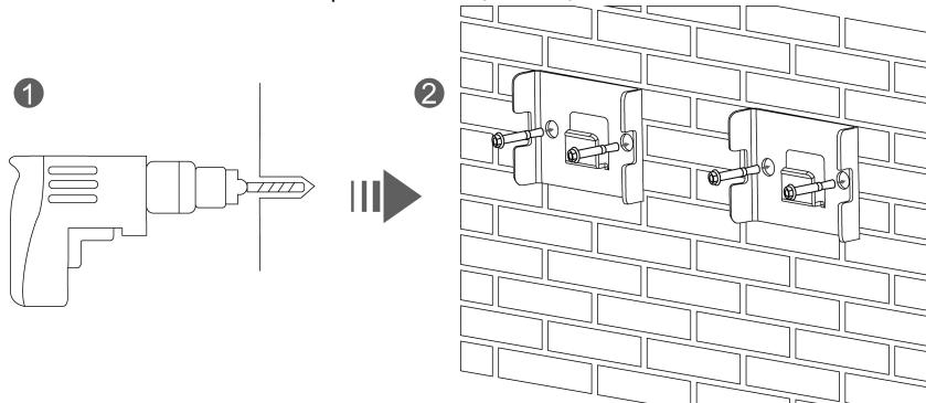
4) Carry the battery and hang it onto the hooks, making sure all bracket mounts on the back of the battery are securely fastened to the hooks on the wall. Secure with two bolts (M4\*12).
