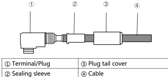
**Overview:** This instruction applies to the terminal crimping installation of the connectors provided in the accessory package. The crimped cable is specifically designed for connection between battery and inverter. Proper installation is crucial to ensure reliable electrical connections and meet protection level requirements. Please strictly follow the steps below.
