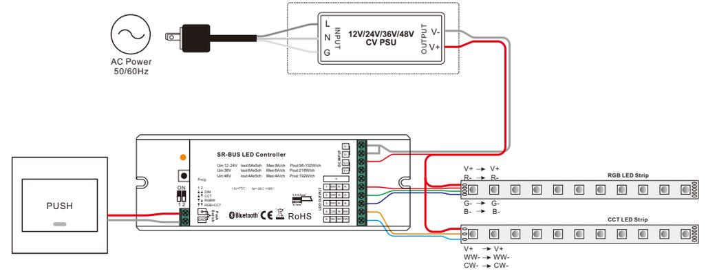
**Note:** please make sure the dial switches are at position for RGB+CCT mode as shown in above diagram.
