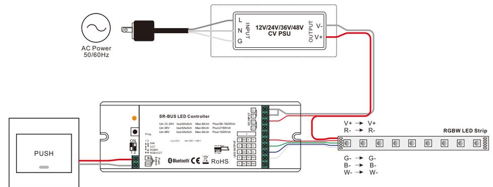
**Note:** please make sure the dial switches are at position for RGBW mode as shown in above diagram.
