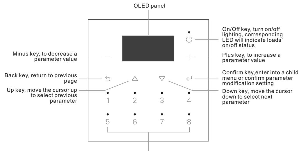
Scene keys 1-8, A. recall corresponding scene, corresponding LED will indicate Loads' on/off status. B. short press scene keys 1-8, DALI scenes 0-7 will be recalled in corresponding control area. B. double press scene keys 1-8, DALI scenes 8-15 will be recalled in corresponding control area. (Please refer to part 3.1.2 "scene saving" to learn how to save corresponding scene parameter.)
