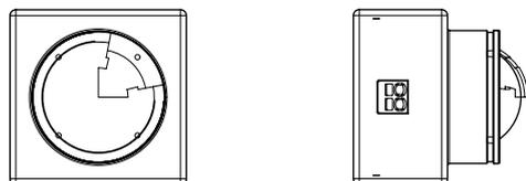
Attach the detection area cover to the sensor by inserting it into the corresponding groove at the front of the sensor.
