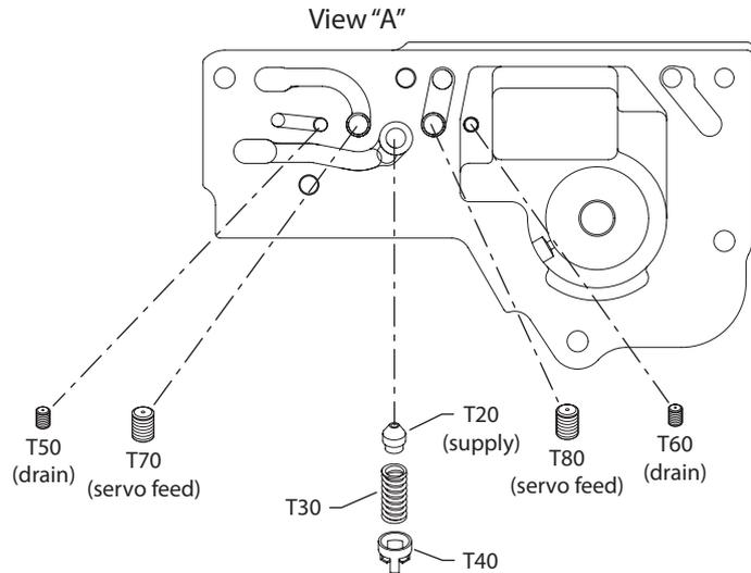
**NOTE:** All orifices present in the original control must be transferred to the replacement control. If replacement control contains pre-installed orifices, remove and discard them before transferring existing orifices to new control.
