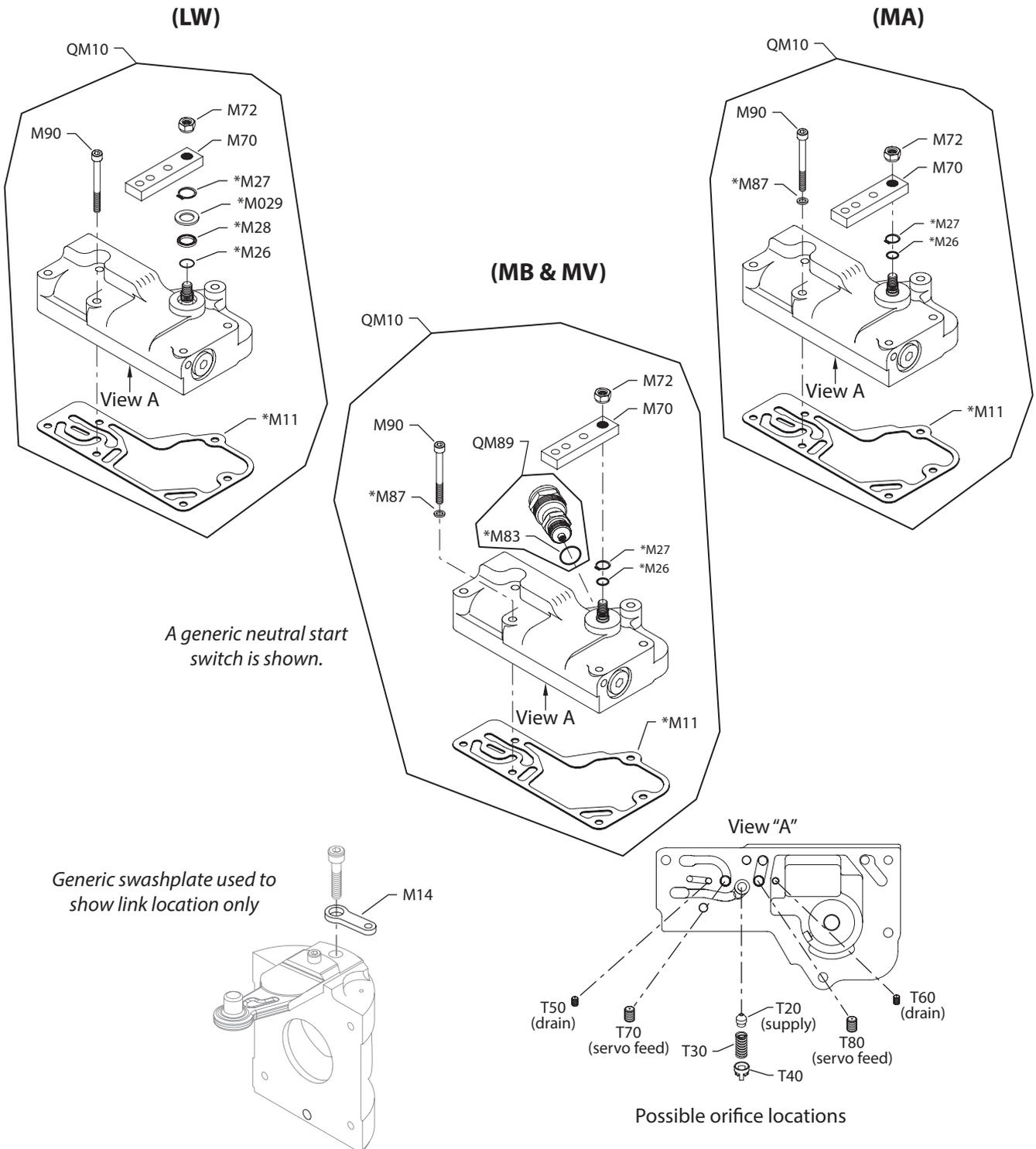
NOTE: All orifices present in the original control must be transferred to the replacement control. If replacement control contains pre-installed orifices, remove and discard them before transferring existing orifices to new control.
