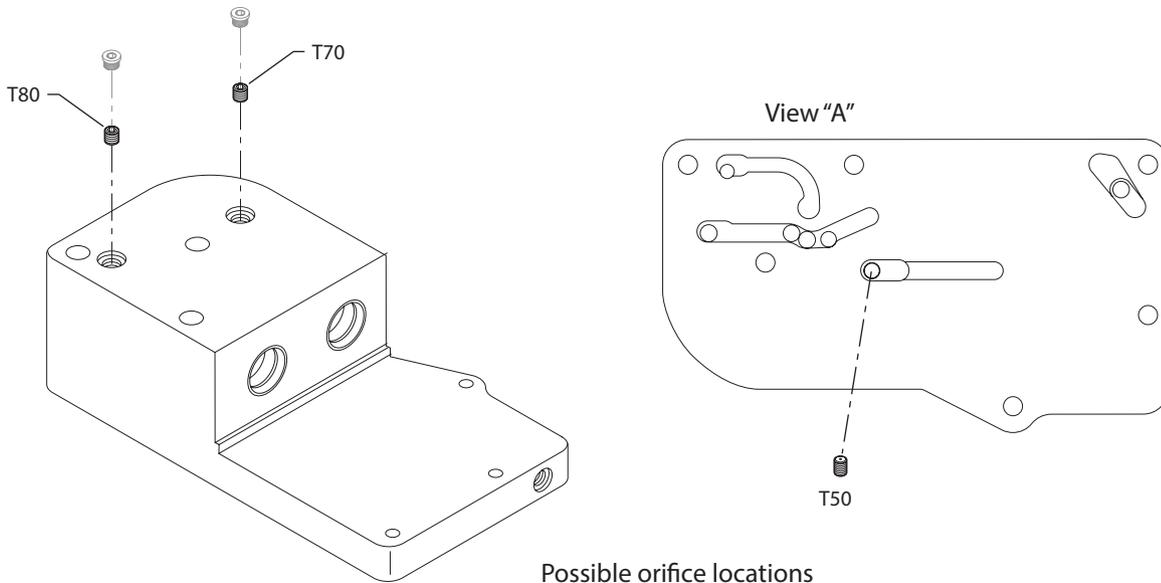
**NOTE:** All orifices present in the original control must be transferred to the replacement control. If replacement control contains pre-installed orifices, remove and discard them before transferring existing orifices to new control.
