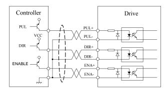
Figure 3: Connections to open-collector signal (common-anode)
