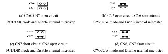
Figure 2:CN6 and CN7 jumper Settings
