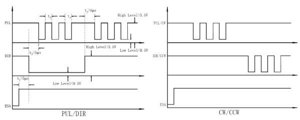
Figure 11: Sequence chart of control signals
