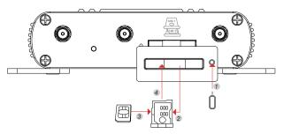
Note: The device is compatible with mini-SIM (2FF) size cards.
