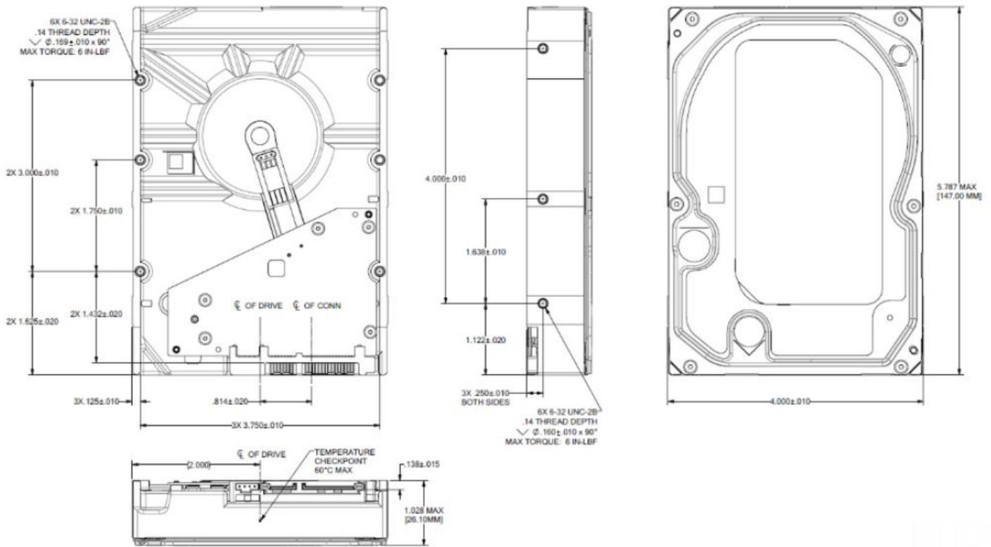
**Figure 5. Mounting configuration dimensions 8TB & 6TB models (Option 2)**
