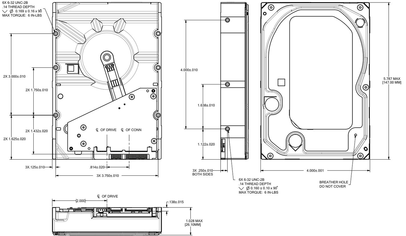
**Figure 4. Mounting configuration dimensions 8TB & 6TB models (Option 1)**
