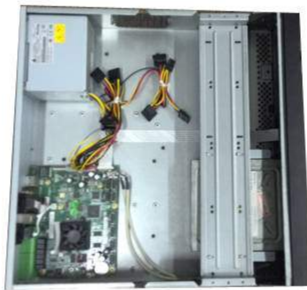
Figure 3-44 Put bracket back
