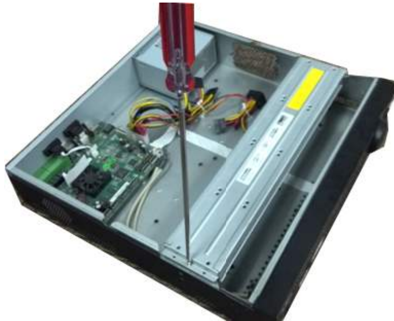
Figure 3-36 Open the top cover
