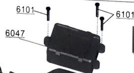
Installation of ESC
