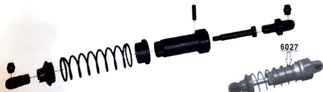
Assembly of the shock absorber
