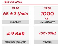
\*The pressure regulator does not function as a bypass.
