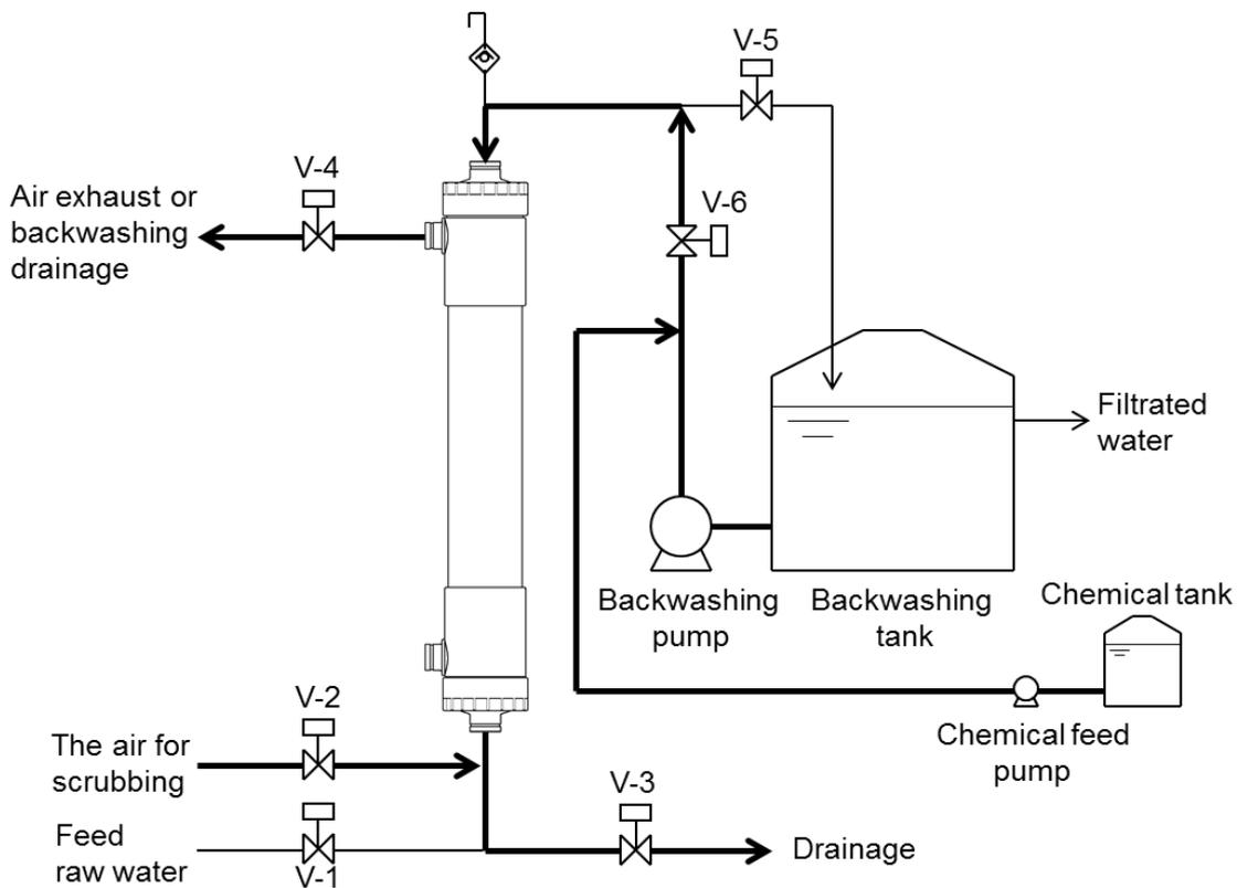
Fig. 4 Flow diagram for backwash and air-scrubbing
