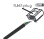
Figure 5.31 Strip the insulation layer and connect to RJ45 plug
