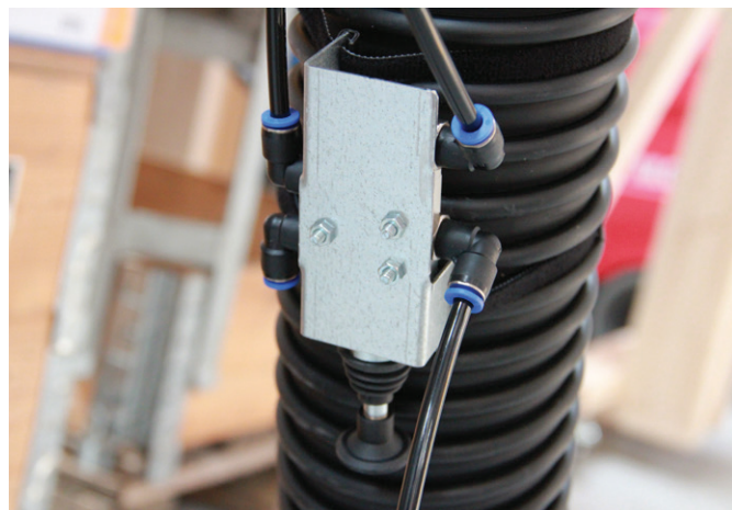
Switch for the pneumatic system
