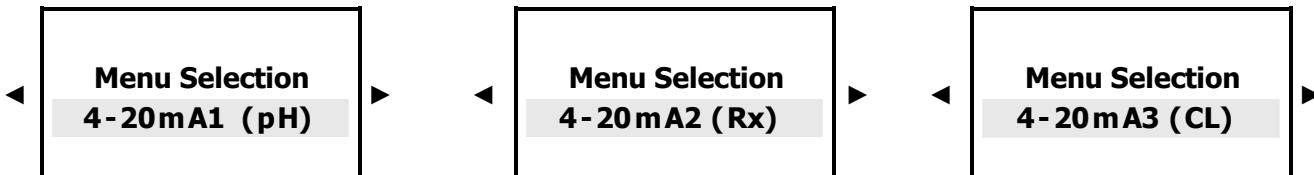
☞ Press **OK/MENU** to go into mA mode. In mA mode the instrument lets you choose two operative functions:
