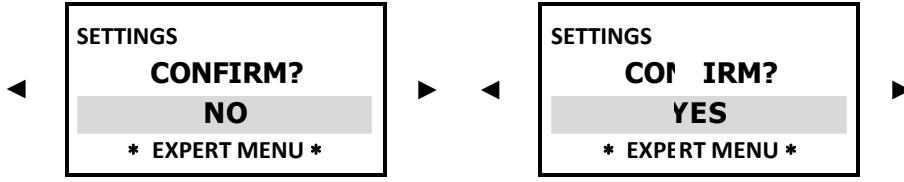
By confirming YES, the display goes out for about 1 second, then goes back to the MEASUREMENT DISPLAY
