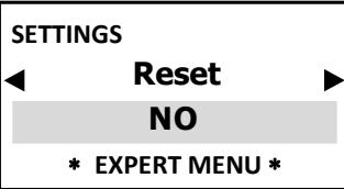
**DATA RESET:** resets default factory settings. ONLY to be used when the parameters do not match or there are programming issues or when the operator wishes to restart from scratch. **NOT** to be overused as many resets may undermine the instrument's efficiency.
