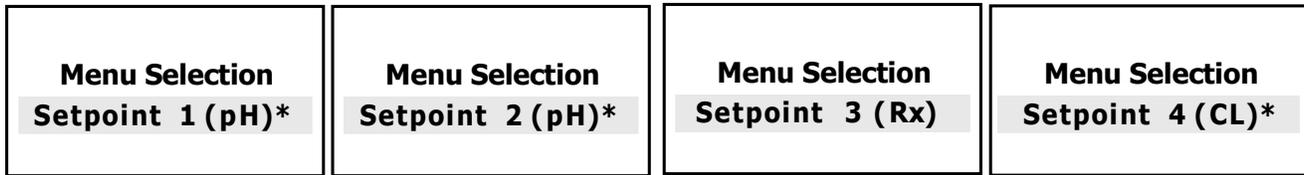
\* By selecting **Measurement Type** **RX**, **SETPOINT1**, **SETPOINT2** and **CALIBRATION** the reading will be RX (mV)
