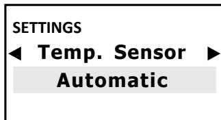
☛ Select AUTOMATIC offsetting for measurements and temperature offsetting with PT100 sensor.
