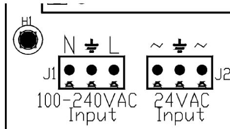
Fig. 1 – Electrical connection
