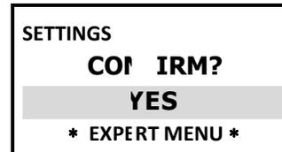
By confirming YES, the display goes out for about 1 second, then goes back to the MEASUREMENT DISPLAY A
