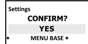
☞ By confirming **YES**, the display goes out for about 1 second, then goes back to the **MEASUREMENT DISPLAY**
