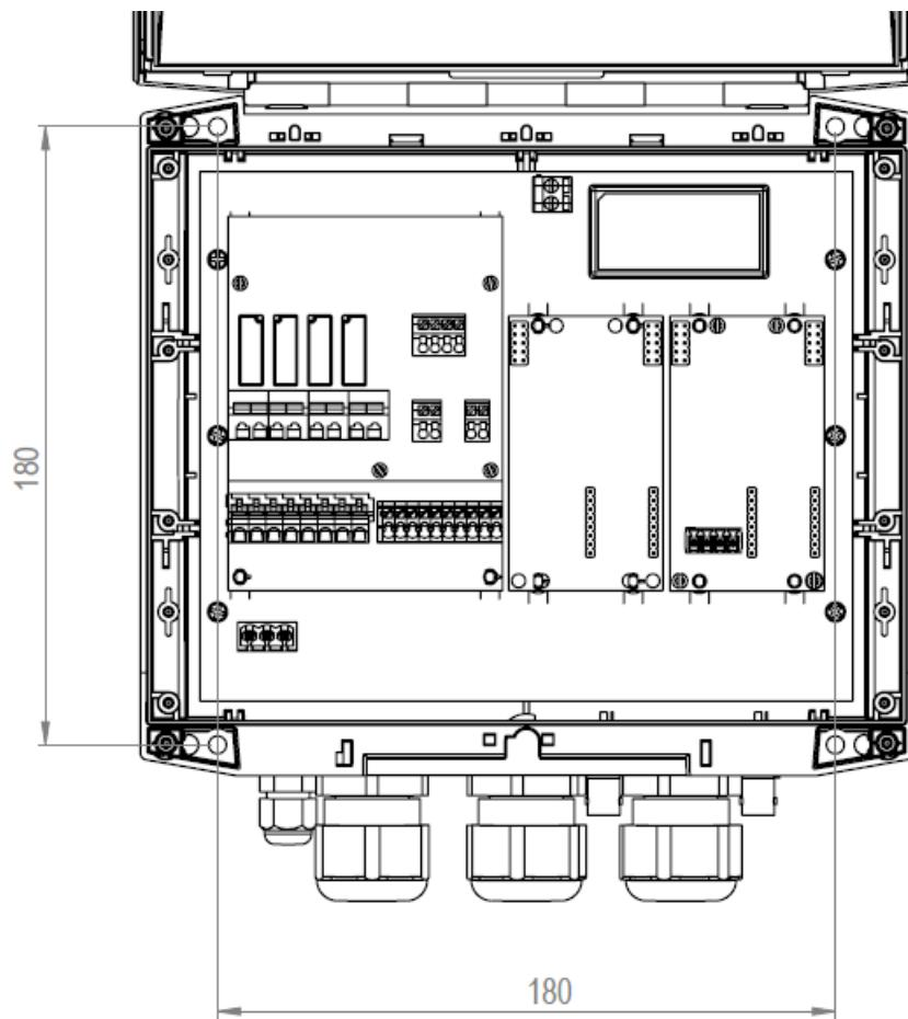
Fig. 2 - Measurements for wall fixing 229l x 204h
