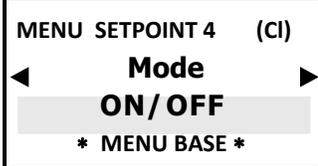
The unit has an **ON-OFF** mode which switches on or off (if the reverse mode is ON) The output relays of Constant / ON-OFF metering pumps or other ON-OFF equipment.
