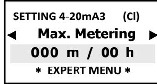
Maximum Metering is a safety function that ensures metering is completed in the selected time. The relays of the metering pumps open accordingly. This function makes it possible to eliminate time limits (continuous metering according to the selected setpoints) or to select the minutes (up to 999) and the hours, for instance metering for 999 minutes in 24 hours.
