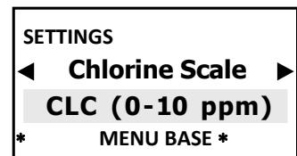
**IMPORTANT:** after selecting the **CHLORINE SCALE**, **ENSURE** the adequate chlorine sensor is connected.
