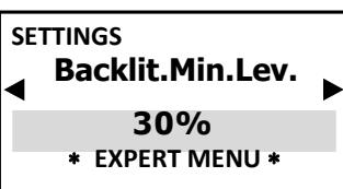
Adjusts display backlighting obtaining energy savings;
