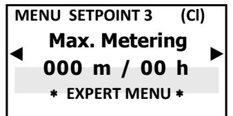
**Maximum Metering** is an extra safety function that ensures metering is completed in the selected time. This function makes it possible to eliminate time limits (continuous metering according to the selected setpoints) or to select the minutes (up to 999) and the hours, for instance metering for 999 minutes in 24 hours.
