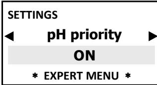
By enabling the pH priority function, the instrument is able to first reach the pH setpoint, then switch to product metering operations (oxidising or reducing agent), thus assuring measurement stability
