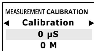
Immerse the EC probe in the buffer solution having a value within the sensor's K range and wait for the measurement to stabilise.
