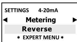
The Direct Dispensing mode means that the output is active when the measured value is lower than the selected setpoint, the connected metering pump dispenses chlorine and vice versa with the reverse mode
