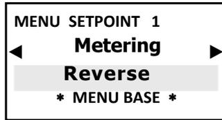
Direct Dispensing Mode: the output is active if the measured value is lower than the selected setpoint, thus activating the connected equipment. The Reverse mode operates exactly in the opposite manner.
