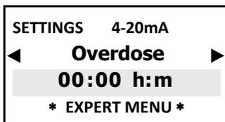
The overdose time-out alarm selects a period of time for reaching the setpoint. If the set point is not reached within the set time, the regulator blocks output operation, including the mA outputs (metering pump). The alarm is displayed ON and activates relay4 activating an alarm device.
