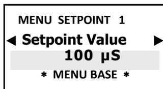
The set point activates the output relays for the metering pumps and other equipment once the selected setpoint level is reached.
