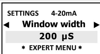
Window width: sets the distance from the set point to the point where the 4-20mA mode is activated: 4 mA = 0 metering pump pulse, 20 mA = max frequency of the metering pump pulses. The window width depends on many variables: distance of the injection point, reaction time, chemical solution %, etc.
