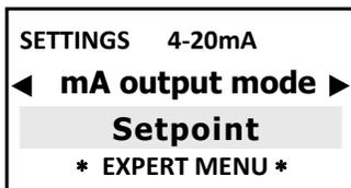
The Setpoint of the proportional 4-20mA analogue outputs follows the setpoint selected below and therefore activates a solenoid valve or metering pump suitable to processing the remote mA current signal.
