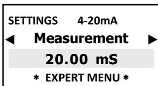
Select the value corresponding to point 20 mA based on **Setpoint 1** settings.
