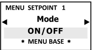
The unit features **ON-OFF mode** which activates (or deactivates in case of reverse mode ON) the output relays as in the metering pump's Constant / ON-OFF modes or of other ON-OFF type equipment.
