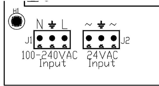
Fig. 1 – Electrical connection
