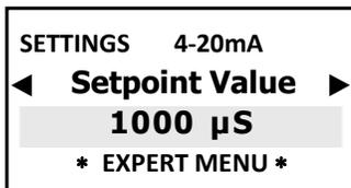
Select the value corresponding to point 4 mA based on **Setpoint 1** settings.
