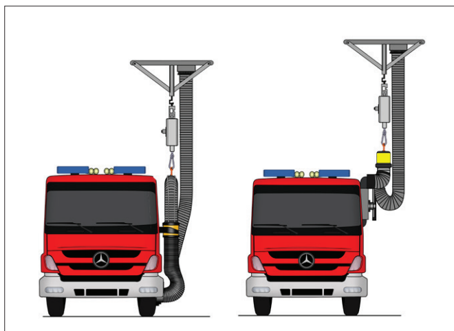
Example with nozzles mounted on exhaust pipes placed low or high
