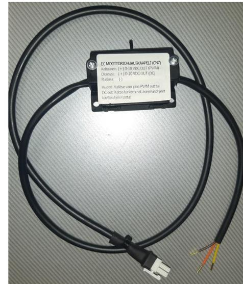
EC connection cable. Connect this always to the CN7 connector of the cooker hood.
