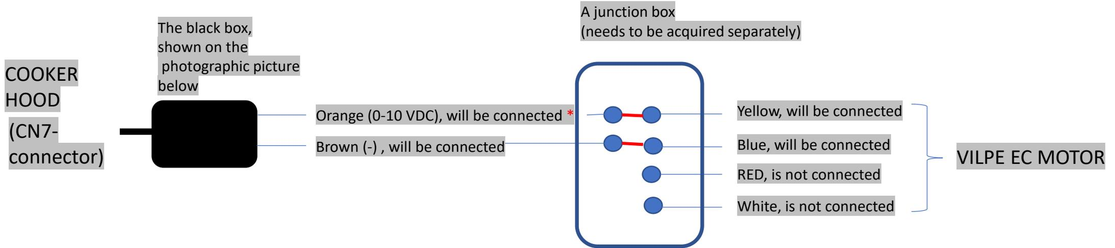
\* = Alternatively you can connect the yellow wire instead of the orange wire. The orange wire provides a flat 0-10 VDC output and the yellow wire provides 0-10 VDC PWM output.
