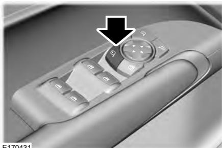
You can fold the mirrors on demand by pressing the power-folding mirror control located on the door. The control lights and the mirrors fold in toward the glass. Press the control again to unfold the mirrors. The control light turns off.
