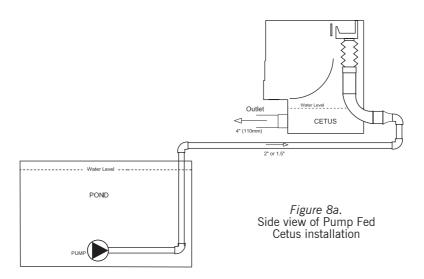
Figure 8a shows the standard way of installing a pump fed Cetus Sieve. While figure 8b shows the way of installing a pump fed Cetus Sieve on a skimmer line.
