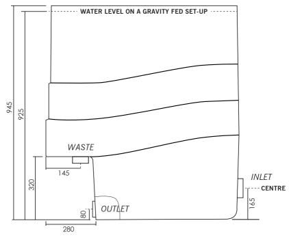
Figure 3a. Cetus Sieve Dimensions (Side View)
