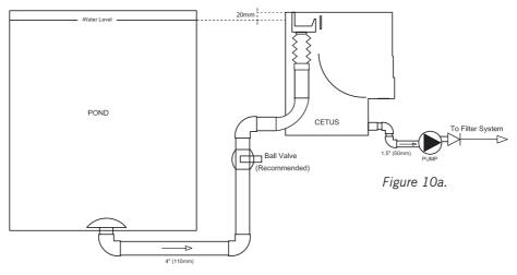
Figure 10a shows the standard way of installing a gravity fed Cetus Sieve. Figure 10b shows a gravity fed installation on a skimmer line.
