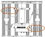
(2) Lock the M4\*12 screw, tighten the bracket for driver
