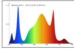
The LED series features a perfect blend of both full-spectrum white LED diodes and red LED diodes. This results in the perfect spectrum for all phases of growth. The mix of white and red LEDs result in a relatively high ratio of bluish light. Blue light keeps your crop tight and compact in the vegetative stage and adds to optimal morphogenesis and light uptake by the plant.
