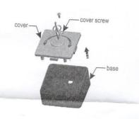
Release the cover screw, turn the key anticlockwise and take out the cover from the base.
