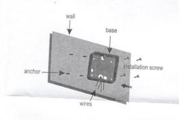
2.Mark the drill points for the base support using the base itself as a reference point. Drill holes in the wall surface for 4 anchors. Fix the base with installation screws in supply. Let wires go through the bottom hole of the base.
