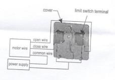
Connect the wires to the terminals of limit switch as the picture, then insert the plastic sheath.
