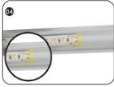
Stick Mylar tape to isolate the cutting position from the bottom of profile inner slot to avoid short-circuit.
