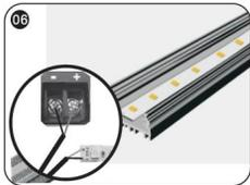
Connect strip wires to the output terminal of the power supply, and dispose with waterproof, insulation, short-circuit, and anti-corrosion protection at wire joints and cut section of your strip (if any).
