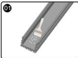
Make sure the mounting surface is clean before installation.
