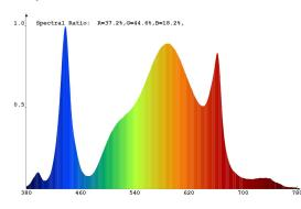
The LED series features a perfect blend of both full-spectrum white LED diodes and red LED diodes. This results in the perfect spectrum for all phases of growth. The mix of white and red LEDs result in a relatively high ratio of bluish light. Blue light keeps your crop tight and compact in the vegetative stage and adds to optimal morphogenesis and light uptake by the plant.
