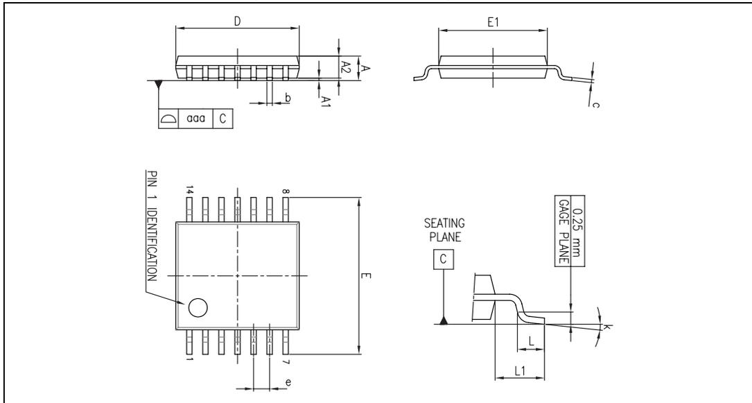
Figure 33. TSSOP14 package mechanical data
