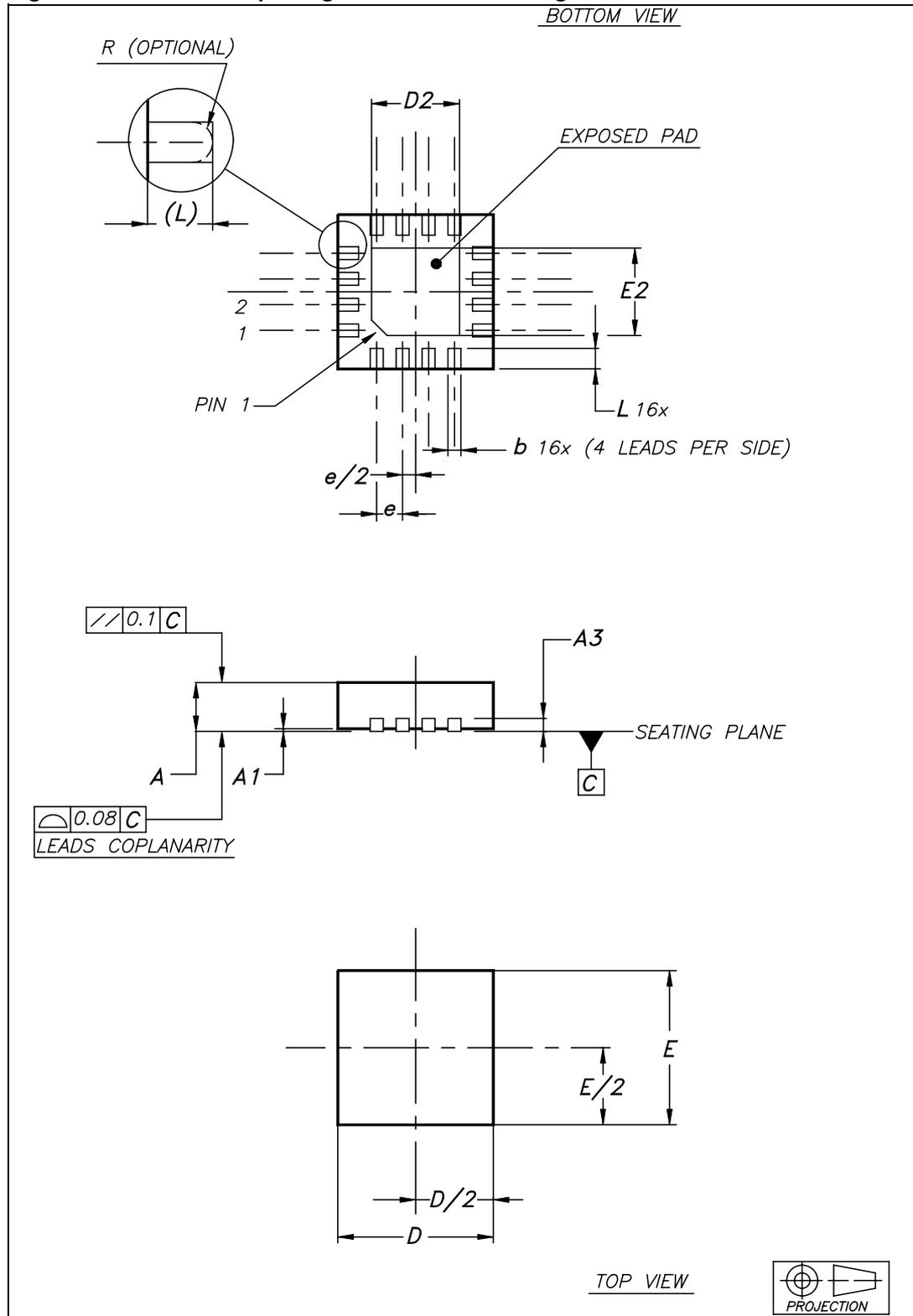
**Table 5. QFN16 3x3 mm package mechanical data (pitch 0.5 mm)**
