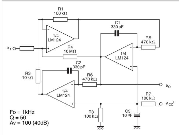
Figure 26. High input Z, DC differential amplifier
