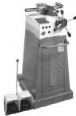
TOP BENDER 050 Maximum capacity 60x4 mm 9040-01-50.
