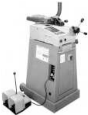
MEGA BENDER 030 Maximum capacity 70x4 mm 9040-01-30
