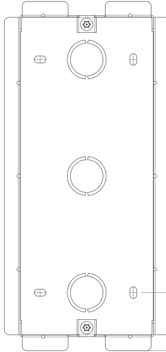
2 FRONT VIEW: FLUSHING MOUNTING BOX PLACEMENT
