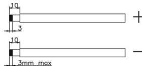
4. Check correct polarity of wire connection from PV modules and PV input connectors. Then, connect positive pole (+) of connection wire to positive pole (+) of PV input connector. Connect negative pole (-) of connection wire to negative pole (-) of PV input connector.
