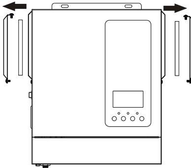
**Step 3:** Clean air filter foam and dustproof case. After clearance, re-assemble the dust-kit back to the inverter.
