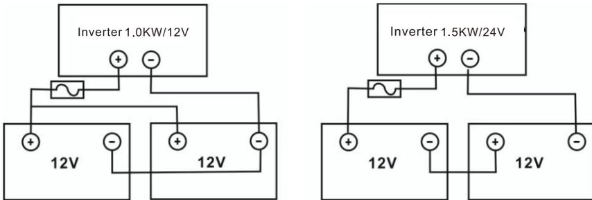
5. Insert the battery wires flatly into battery connectors of inverter and make sure the bolts are tightened with torque of 2 Nm in clockwise direction. Make sure polarity at both the battery and the inverter/charge is correctly connected and conductors are tightly screwed into the battery terminals.
