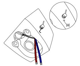
7.Install the handle (G) on A, tighten it with a 7-character wrench(F), and cover it with a decorative cover(H).
