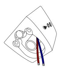
4.Install the black rubber gasket (B+C) and tighten it
