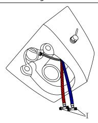
8. The inlet angle valve(I) one side connected with the cold/hot water pipe and another side connected water inlet pipe
