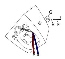
6.Screw the screw (E) to the handle (G) with a 7-character wrench(F).
