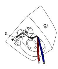
5. Tighten the nozzle water inlet pipe(D) after connecting it to the washing nozzle
