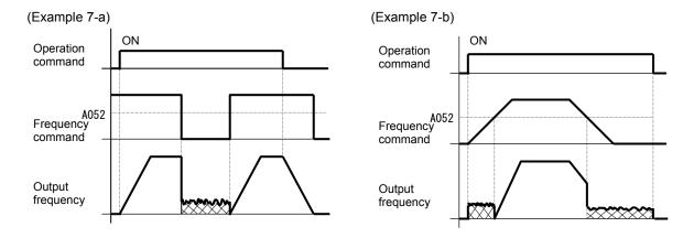
How the inverter returns to the normal output varies depending on the setting of the DC braking/edge or level detection for [DB] input (A054).
