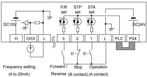
\* This wiring diagram is an example of using the built-in power inverter. Refer to Section 5.6, when you use an external power supply.
