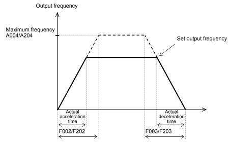
The actual time to accelerate/decelerate the motor will be no less than the minimum acceleration/deceleration time that depends on the inertial effect (J) due to the mechanical system and motor torque. If you set a time shorter than the minimum acceleration/deceleration time, the inverter may trip because of overcurrent or overvoltage.
