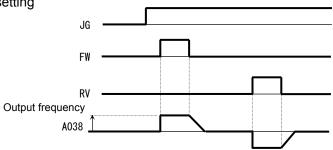
Since the inverter operates the motor with a full voltage for the jogging operation, the inverter can easily trip during the latter. Adjust the jog frequency setting (A038) properly so that the inverter will not trip.
