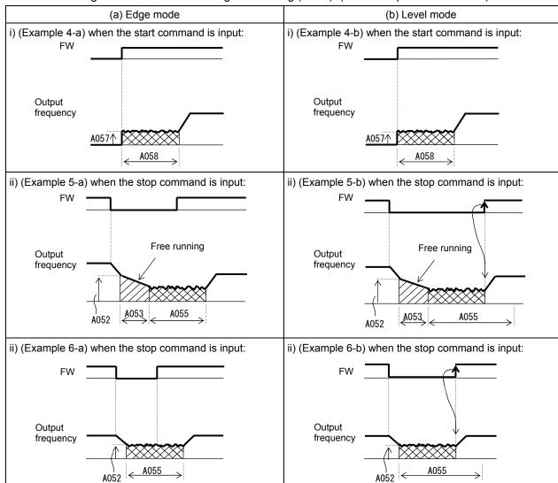
(4) Internal DC braking (triggered only when the output frequency reaches a set frequency) (A051: 02) You can also operate the internal DC braking function so that DC braking is applied to the motor when the inverter output frequency falls to the DC braking frequency setting (A052) or below.
