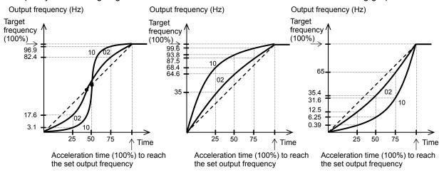
The acceleration or deceleration time may be shortened midway through the acceleration or deceleration according to the curve pattern.
