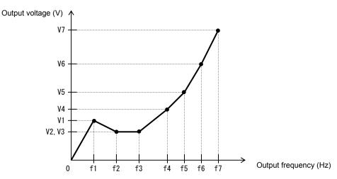
\*1 Even if 300 V is set as a free-setting V/f voltage (1 to 7), the inverter output voltage cannot exceed the inverter input voltage or that specified by the AVR voltage select.
