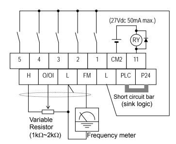
Note1)The above is a method to perform analog input(O/OI) by voltage input. It is necessary for SW6 on the board to be set for voltage input(default).
