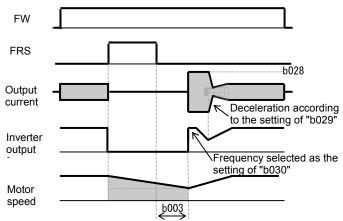
After the retry wait time (b003), the inverter restarts the motor with the frequency set as "b030". The inverter subsequently decelerates the motor according to the setting of "b029" while maintaining the output current at the level specified for "b029". When the output voltage matches the frequency, the inverter re-accelerates the motor up to the frequency that was set when the inverter shut off the output to the motor before the restart
