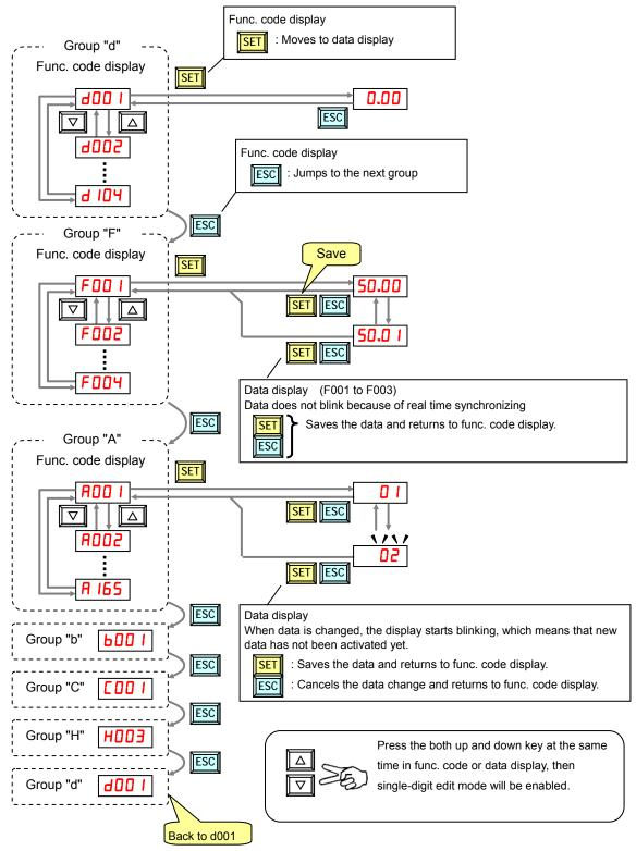
Note) Pressing the [ESC] key will make the display go to the top of next function group, regardless the display contents. (e.g.  $ROZ I \rightarrow [ESC] \rightarrow bOO I$ )
