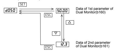
Note) If it enable the Frequency set in monitoring( $\frac{163}{0}$ ), ( $\frac{1}{0}$ ) and ( $\frac{1}{0}$ ) can change the output frequency as per  $\Delta \nabla$  key in driving. But ( $\frac{1}{0}$ ) can not chang ( $\frac{1}{0}$ ) and ( $\frac{1}{0}$ ).
