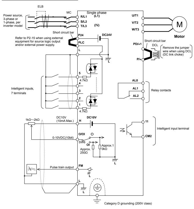
Note 1) Above shows an example of voltage (O) input. Changeover of SW6 must be done in case of current (OI) input.
