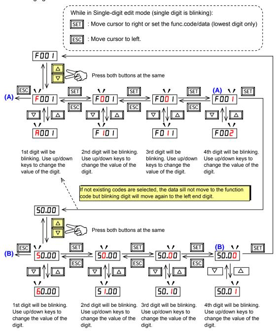
Note1) When pressing [ESC] with cursor on the highest digit, the cursor will jump to the lowest digit. ((A) and (B) in above figure.)
