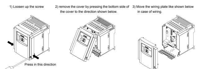
Screw for fixing the front cover is located at right-bottom side
