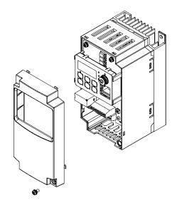
3) The connector of the exclusive operator (NES1-OP) connect to the connector on the circuit board. And attach it to put the circuit board.
