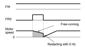
The inverter restarts the motor with 0 Hz regardless of the motor speed. The setting of retry wait time is ignored.
