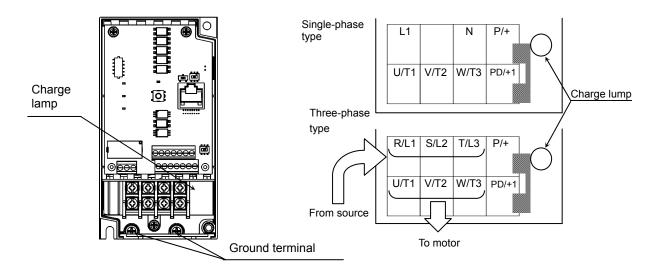
Single-phase 200V 0.75 to 2.2kW Three-phase 200V 1.5, 2.2kW
