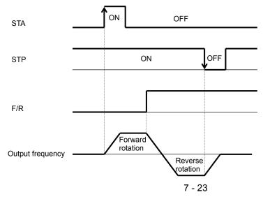
Note: In 3 wire input, STP input is used at the b point of contact.
