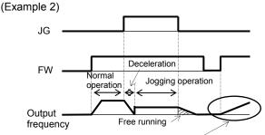
Acceleration according to the setting of "b088"
