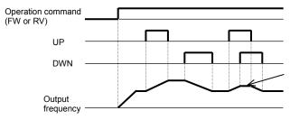
Turning on the UP and DWN terminals at the same time disables acceleration and deceleration
