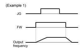
When "00", "01", or "02" is specified for the jog stop mode (A039), the jogging operation will not be performed if the FW signal is turned on earlier than the JG signal.
