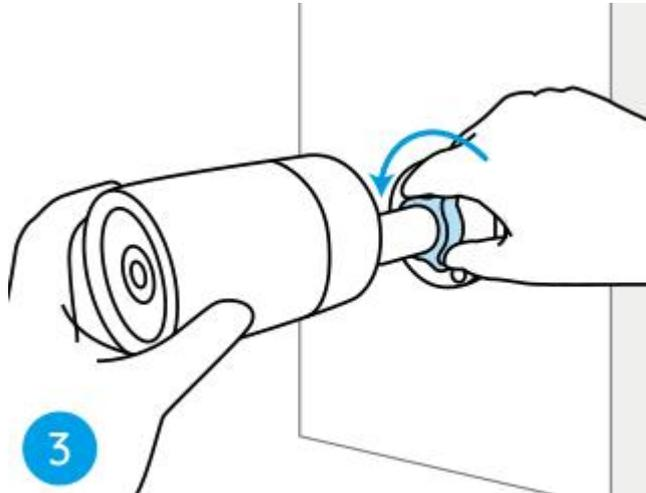
**Step 4.** Turn the knob clockwise to fix the camera in place.
