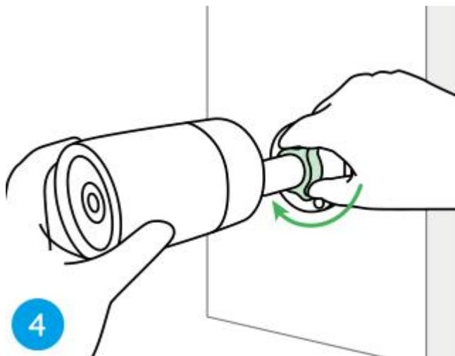
**Note:** If your camera has another mount without the adjusting knob, please loosen the adjusting screw with the provided hex key and turn the camera as shown below to adjust the angle.
