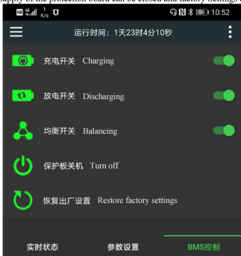
Figure 34. The BMS control page
