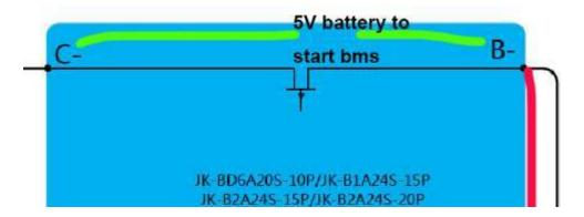
C. open the bms case, then use the charger to start the bms as below pic show This way no need battery, use the charger positive and negative wire connect to bms + and – as pic show (donot advise this way for safe reason)
