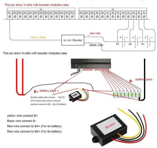
12v battery, use 12v to 48v booster, 24v battery use 24v to 48v booster.
