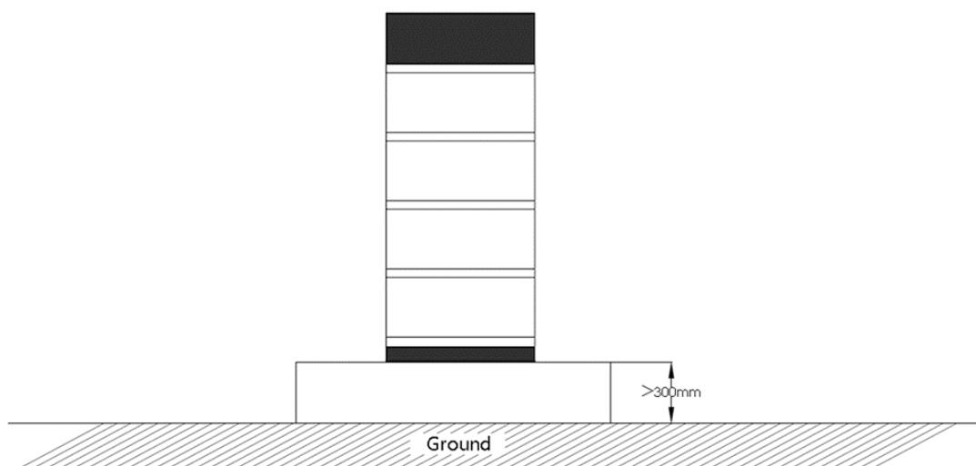
**NOTE** The above illustration is just for reference. The quantity of the battery modules is based on your practical system.
