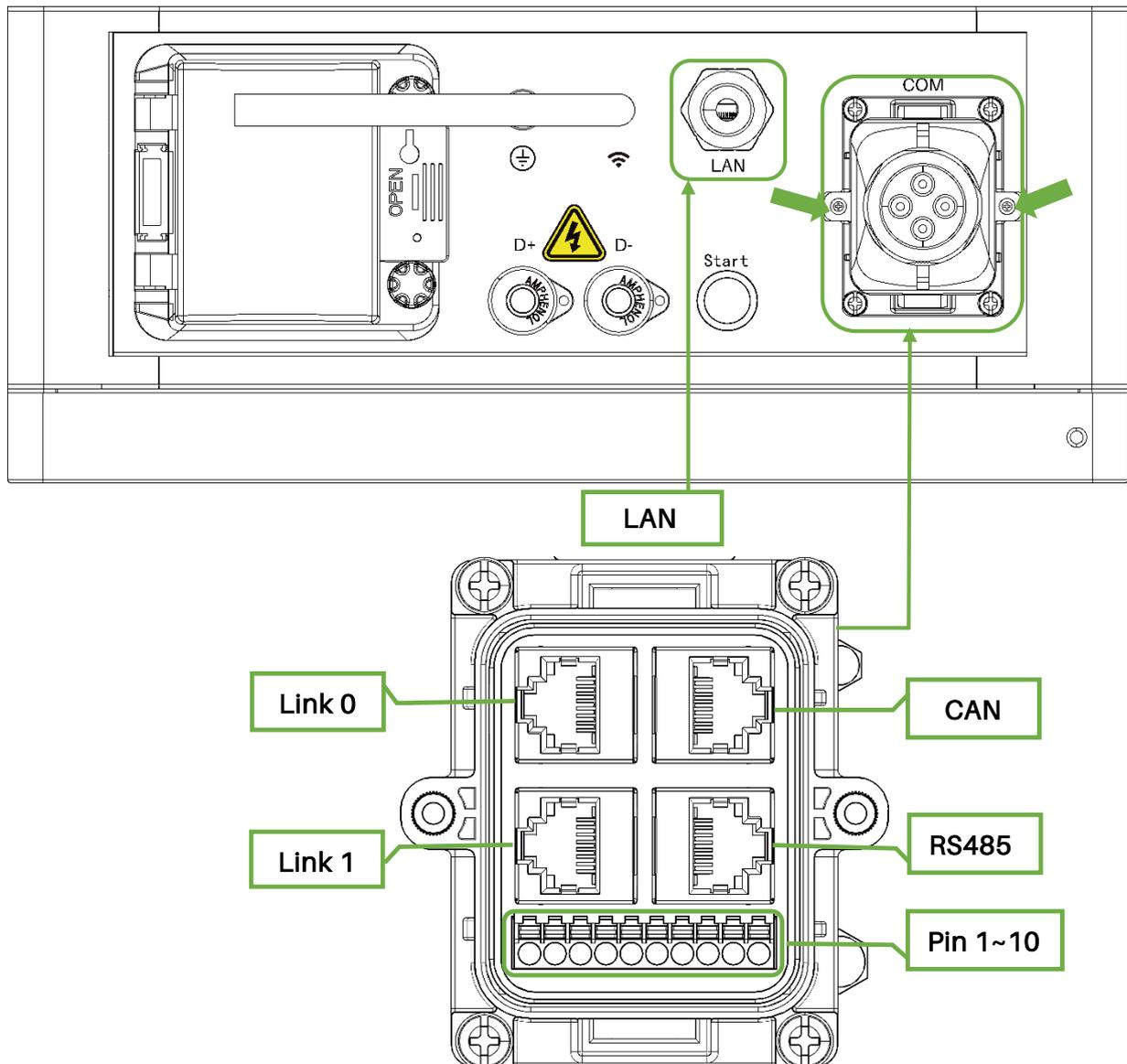
**LAN:** Used for where the Wi-Fi signal is not good or there is no Wi-Fi. To connect to the online portal directly through a network cable (another side to the internet router).
