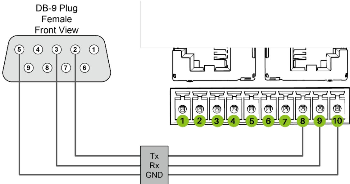
For communication cables connection for PIN1~10 terminal station, please follow the steps below:
