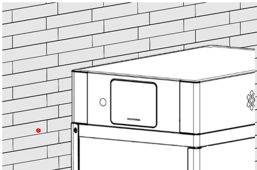
6. Embed the two M8 expansion bolts into the holes respectively.
