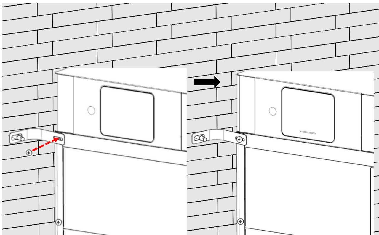
8. Fix the M8 nut (a) across the 8mm flat gasket (c) and spring washer (b), with 12~13N.m torque. Repeat this step for the other bracket.
