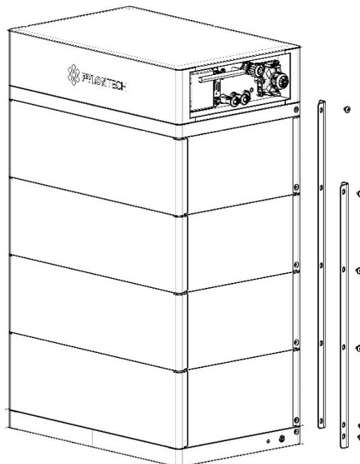
6. Remove the control module and each battery module one by one.
