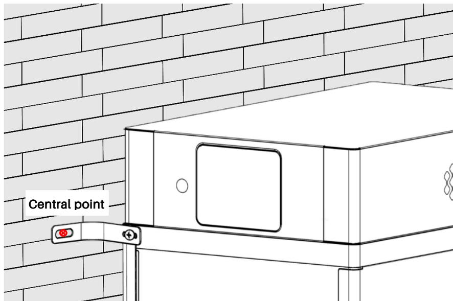
5. Dismantle the brackets on both sides. Aligning the central points, drill two holes ( $\geq 60\text{mm}$  depth) in the wall with a drilling tool, and clean the holes.
