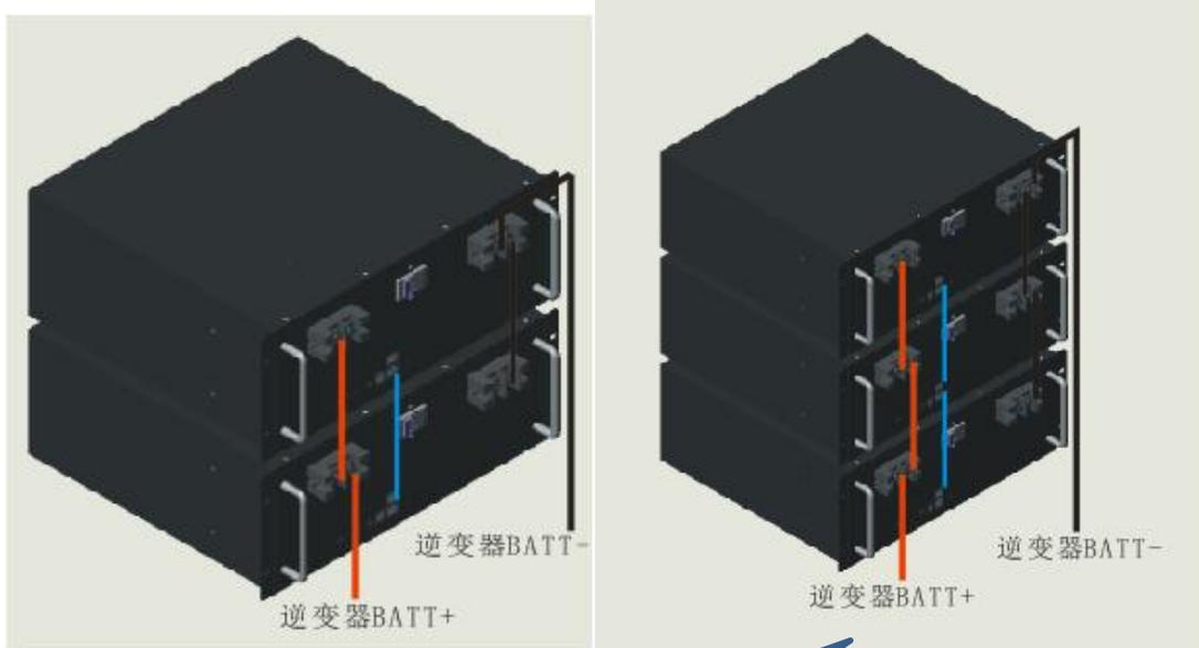
Note: when connecting the equipment, the battery output positive and negative electrodes should be taken from the first group and the last group of batteries
