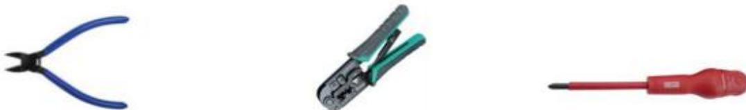
Use insulated tools to prevent accidental electric shock or short circuit. If there is no insulation tool, use insulation tape to cover all exposed metal surfaces of the tool for insulation treatment.
