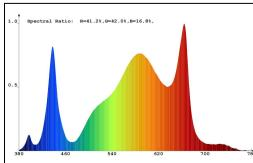
The LED series features a perfect blend of both full-spectrum white LED diodes and red LED diodes. This results in the perfect spectrum for all phases of growth. The mix of white and red LEDs result in a relatively high ratio of bluish light. Blue light keeps your crop tight and compact in the vegetative stage and adds to optimal morphogenesis and light uptake by the
