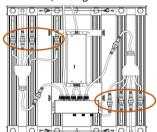
(2) Lock the M4\*12 screw, tighten the bracket for driver
