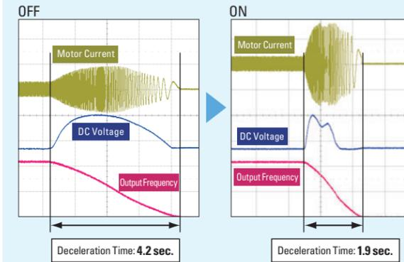
2.3 sec. reduction of deceleration time without a braking resistor is achieved when the function is active.
