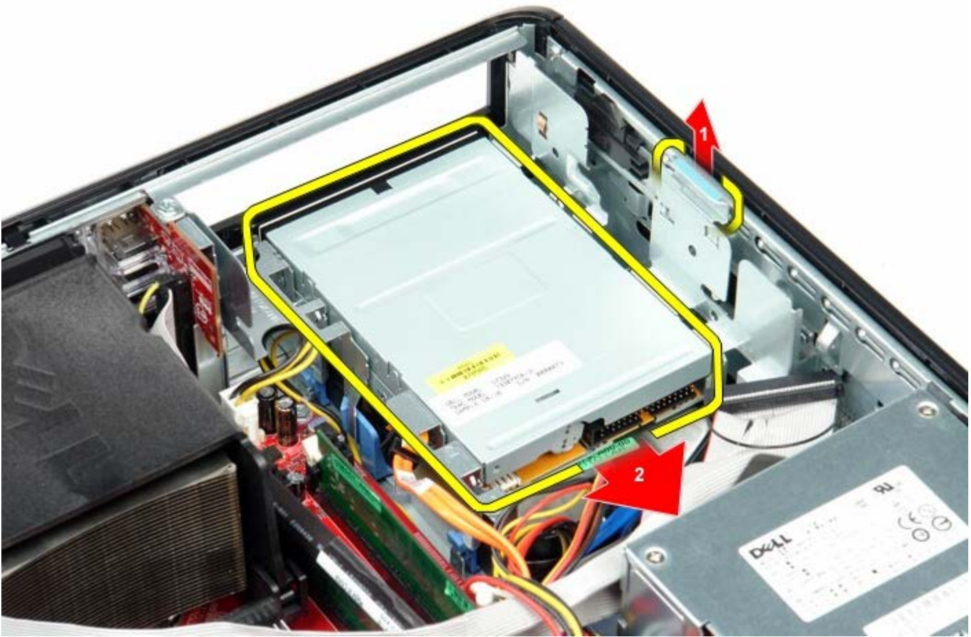
5. Lift the floppy drive up and away from the computer.
