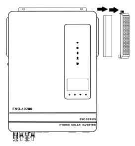
**Step 3:** Clean air filter foam and dustproof case. After clearance, re-assemble the dust-kit back to the inverter.
