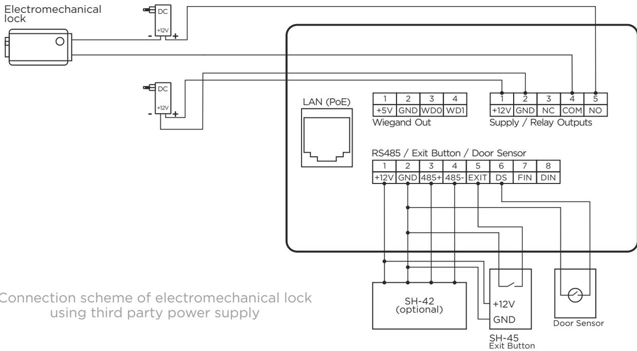
Connection scheme of electromechanical lock using third party power supply
