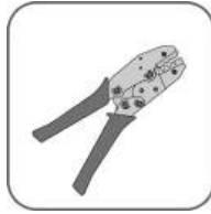
Tube terminal crimping tool (0.5 mm 2 – 1.0 mm 2 )
