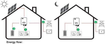
$PV \rightarrow Load \rightarrow Grid \rightarrow Battery$
