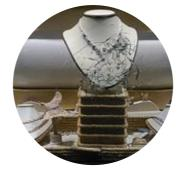
Clear 7 C films help secure your windows by ensuring that the glass does not shatter, remaining transparent and retaining its overall integrity in the event of an impact, explosion or fire. Comply with European Standard EN 12600.
