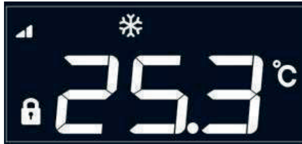
Cooling in smart mode main interface
