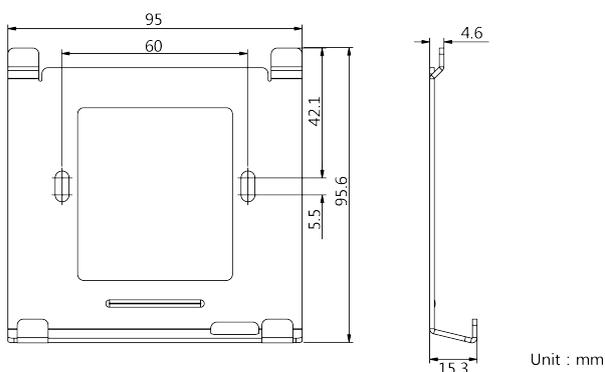
Figure 5-1 Wall Mounting Plate
