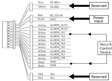
Figure 4-1 Wiring Description (Alarm Input Device)
