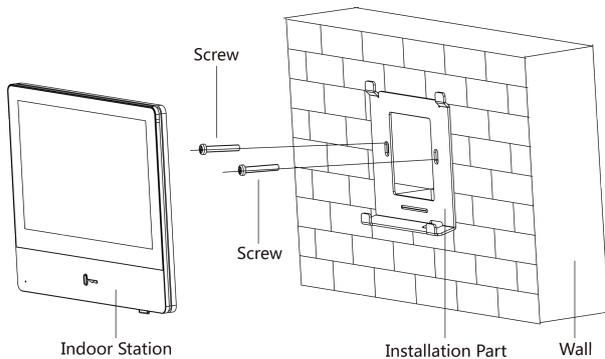
**Figure 5-2 Installing the Plate**
