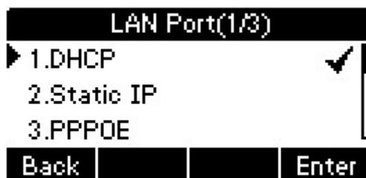
3. Press soft key Enter or OK button to enter the DHCP setting interface,after obtain the IP address,it will automatically back to the previous interface
