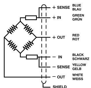
«SENSES»: 2 additional wires to maintain a constant voltage supply at the load cell when used with proper instrumentation. Use especially when long wires and wide temperature range.
