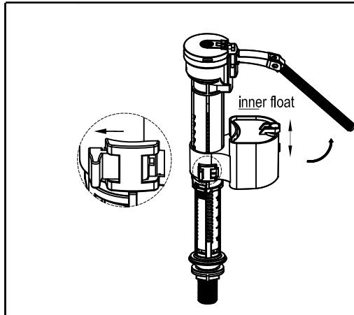
3. Install fill valve into tank
